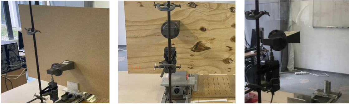
Figure 4.19 Experimental system for microwave broadband free-space sensing. Different planar MUT in front of the horn antenna.
