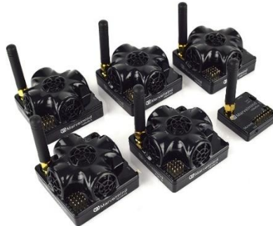
Figure 2.3 Modem and Beacons of the Marvelmind Indoor Navigation System.
