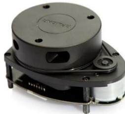
Figure 2.2 2D LIDAR - RPLIDAR.
