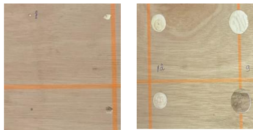
(a) Circular cracks
