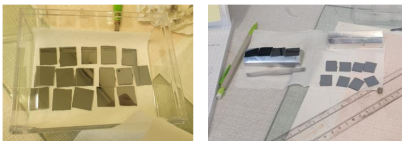
Figure 93: left) Silicon wafer pieces of 1.6 \times 1.8 \text{ cm}^2 and right) pieces placed in the support for polishing.
