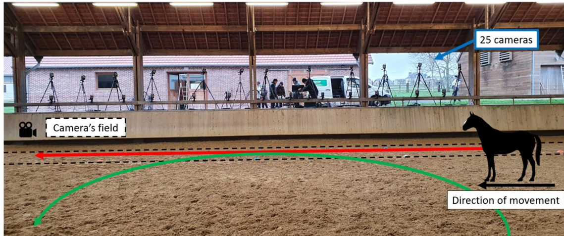
Figure 27 : Positioning of the Vicon cameras on one side of the indoor arena. The black dotted lines correspond to the camera's field. The trajectory of the straight line during walking and trotting is represented by the red arrow, and the trajectory of the circle during galloping is represented by the green arrow.
