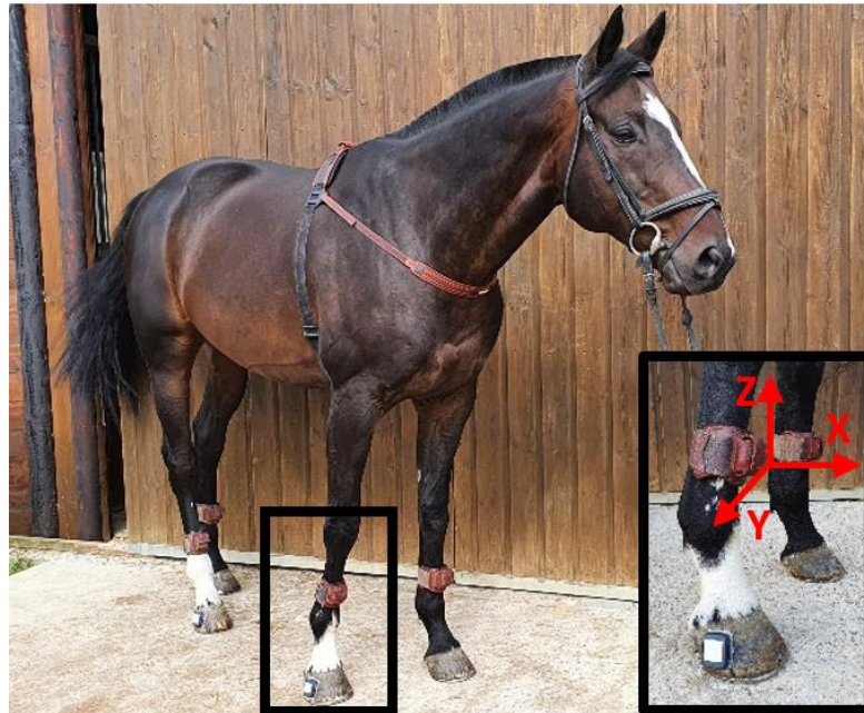
Figure 18 : IMUs localization on horse: on the withers, on the four limbs, in the center of the dorsal side of the third metacarpal bone (cannon bone), and on the lateral quarter of the right front and hind hoof.
