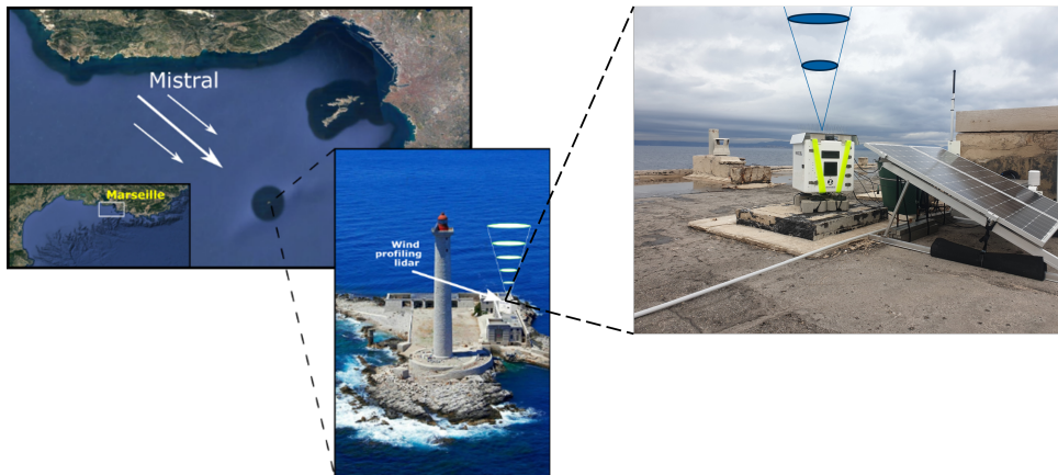
Figure I.7 – The Planier LIDAR operated by France Energies Marines installed on the Planier island for the recording of long-term time series of offshore wind profiles.
