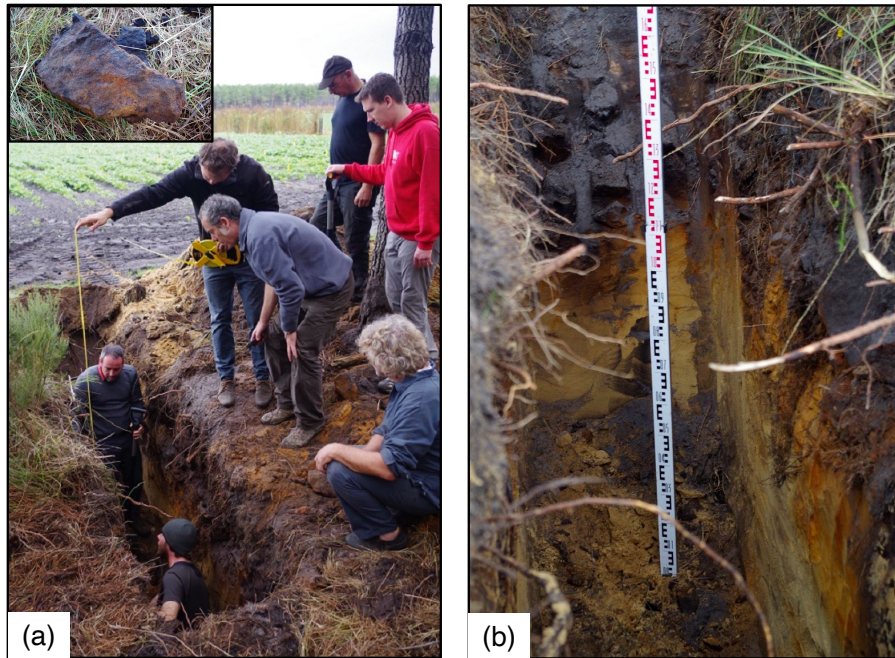
Figure 2.3: (a) Soil pit locally excavated down to 2.5m at the edge of the forest reveals a highly compacted sand interface called “alios” (see inset). (b) This compacted sand layer is located approximately from \sim 0.5\text{m} to 1.5\text{m} below the surface and is ploughed before plantation, particularly to allow water percolation into the ground. The ground water table was approximately 1.7\text{m} from the surface during the experiment. The same subsurface structure has been observed both in the forest and the field, except for the parallel row structure and presence of tree roots in the forest. (Images are accessed from metaforet.osug.fr )
