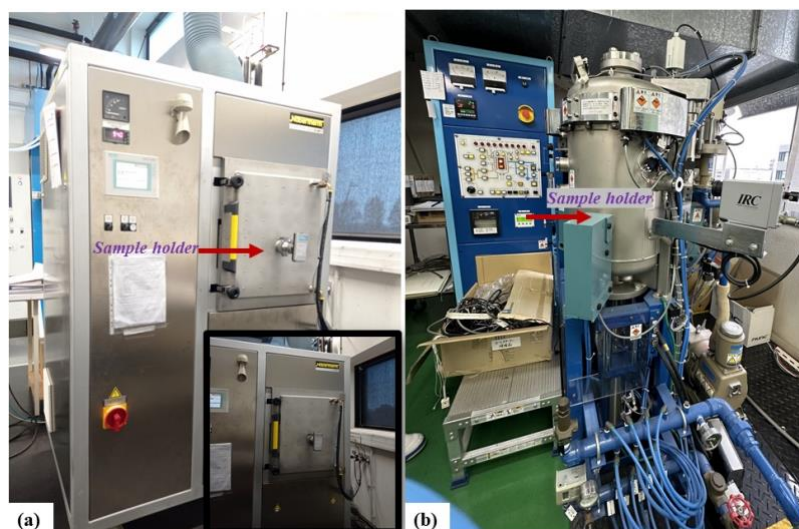
Figure II.7. (a) Graphite furnace for heat-treatment 9 (b) GPS Sintering furnace 10 .
