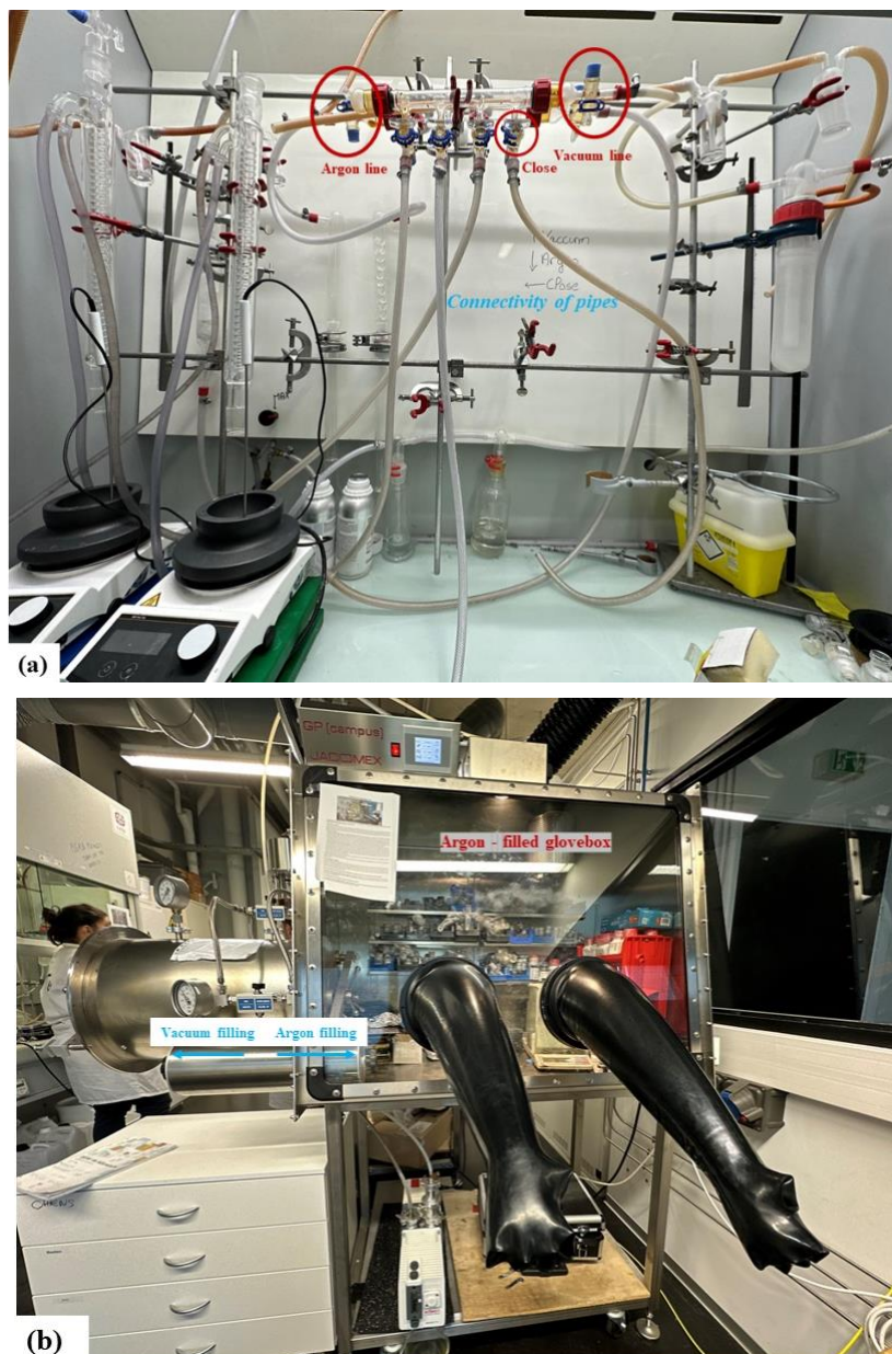
Figure II.1. (a) Schlenk line for synthesis experiments and (b) argon-filled glovebox for precursor manipulation.
