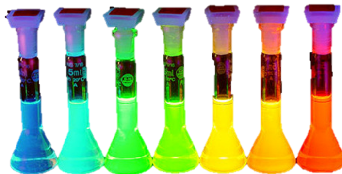
Figure 1.7: Fluorescence of CdSe-CdS nanoparticles with diameters varying from 1.7 nm (blue) up to 6 nm (red). Reproduction by H. Weller, University of Hamburg. Taken from Ref. [34].
