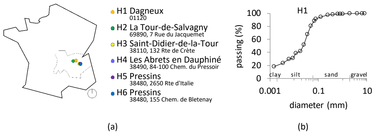
Fig. 3.1: (a) Situation of the collected rammed earth materials; (b) Particle size distribution of H1 rammed earth.
