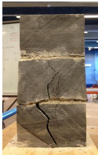
Figure 8: Sample of a schist triplet after failure.
