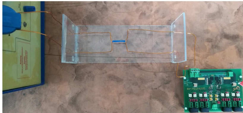
Figure 3.20: Dedicated setup for power wires between LISN and converter input. It keeps 2.5 cm distance of the power wires to the ground and provide comfortable connection of current probe at the constriction
