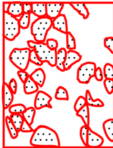
Figure 3.21: Superposition of the outline of the GaN domains with the map of pillars (seen as black points) having a pitch of 1.5 μm and distributed a hexagonal pattern.
