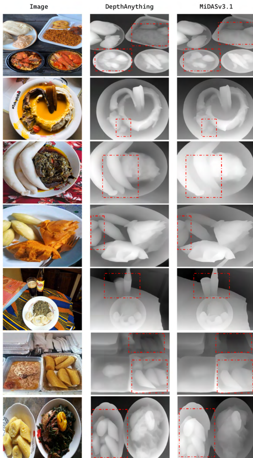
Fig. 5.18 Qualitative comparison between the MiDASv3.1 and DepthAnything models on zero-shot relative depth estimation of some image from the CamerFood15 dataset.
