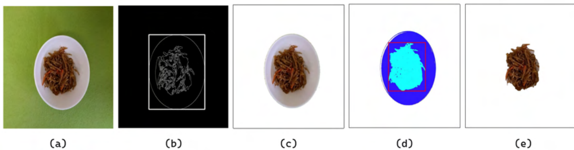
Fig. 3.8 The processing steps of food region extraction proposed by Okamoto et al.. (a) Provide a meal photo, (b) Detect a bounding box of a food dish region based on edges, (c) Detect a bounding box of food region by k-means, (e) Detect food region by Grabcut.
