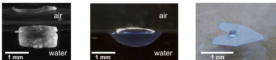
Figure 1.2: Types of Marangoni swimmers. Examples of the different types of Marangoni swimmers, from left to right: aspirin [23] (dissolving swimmer), polyethylene glycol in alginate capsule [25] (loaded swimmer), aluminum-ethanol [29](boat).
