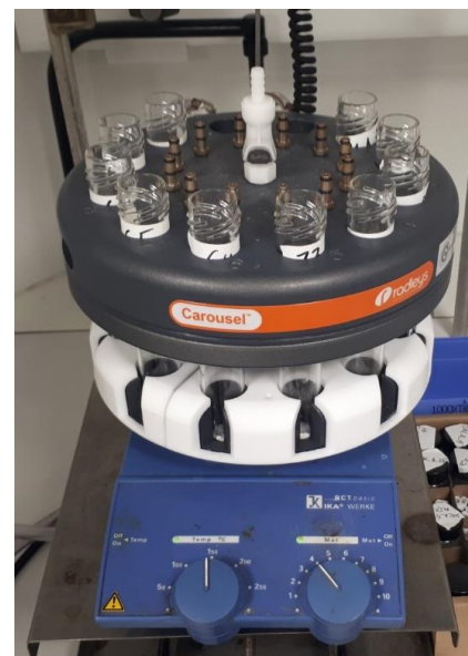
Figure 46. Radleys Carousel 12 Plus Reaction Station for studying the scope of prebiotic reactions
