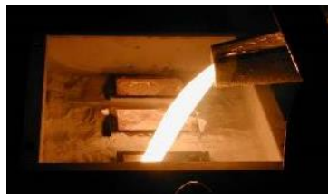
Figure 111: Pouring in the moulds.
