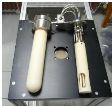
Figure 36: Sample holder of the conductivity set-up.
