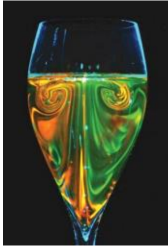
Figure 1: Illustration of the convective movements enhanced by the blistering in a champagne glass as a comparison of the stirring phenomenon in a glass furnace [15].
