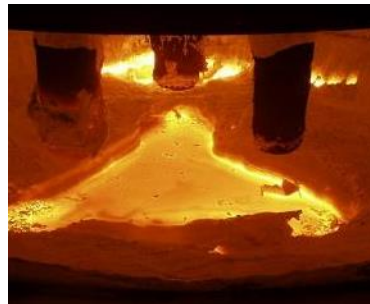
Figure 110: Fusion with the three graphite electrodes.
