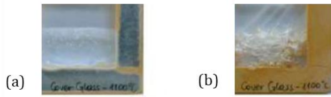
Figure 22: Self-crucible test for (a) raw HZB and (b) pre-oxidized HZB refractories at 1100°C in contact with cover glass for 30 hours at air atmosphere [63].
