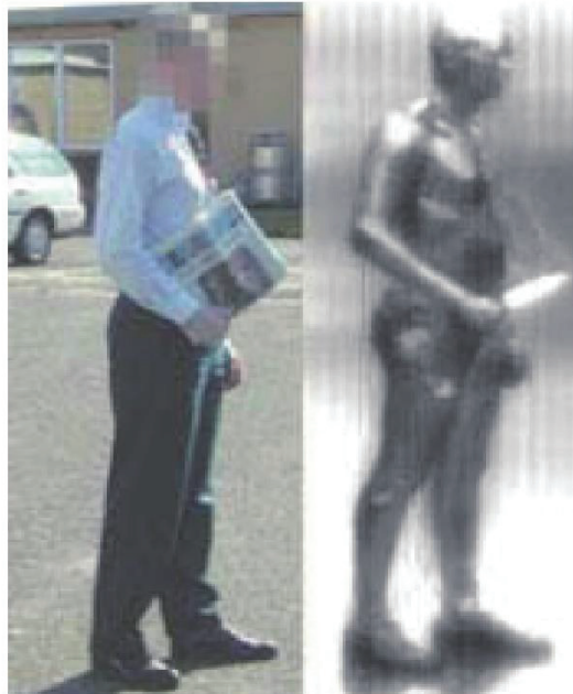
Figure. 5.1.2. Image obtained with a terahertz human security scanner for the detection of hidden dangerous goods.
