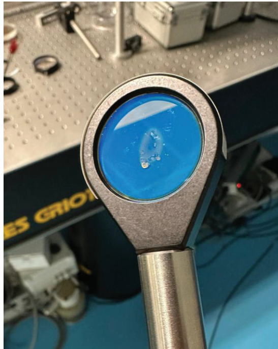
Figure 4.2.10. Phase plate damaged by the laser with high peak power. Laser energy was 100 mJ and pulse duration was 300 fs.
