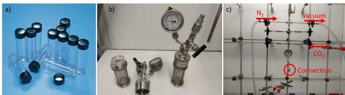
Figure 3: Typical equipment used for adsorption reactions. a) Vials, b) autoclaves, c) gas system.
