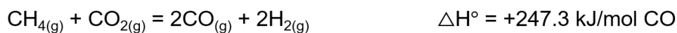
Figure 2: Standard enthalpy of reaction associated to steam reforming and dry reforming of methane.
