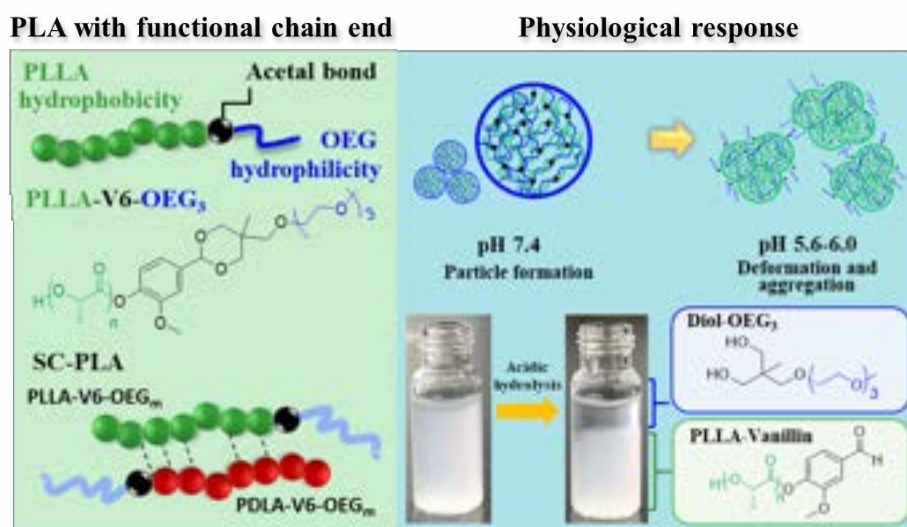
Figure 1-17. Preparation of PLA with functional chain-end via functionalized initiator.
