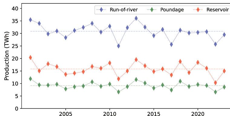
Figure 1.2: Annual production by hydropower plant type (RTE, 2023a).
