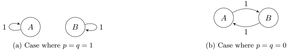
Figure 3.1: The two different configurations where |p + q - 1| = 1 . On the left, p = q = 1 . This means whatever the initial configuration, the edge will stay in the same state. On the right, p = q = 0 . This means the edge state changes at every step.
