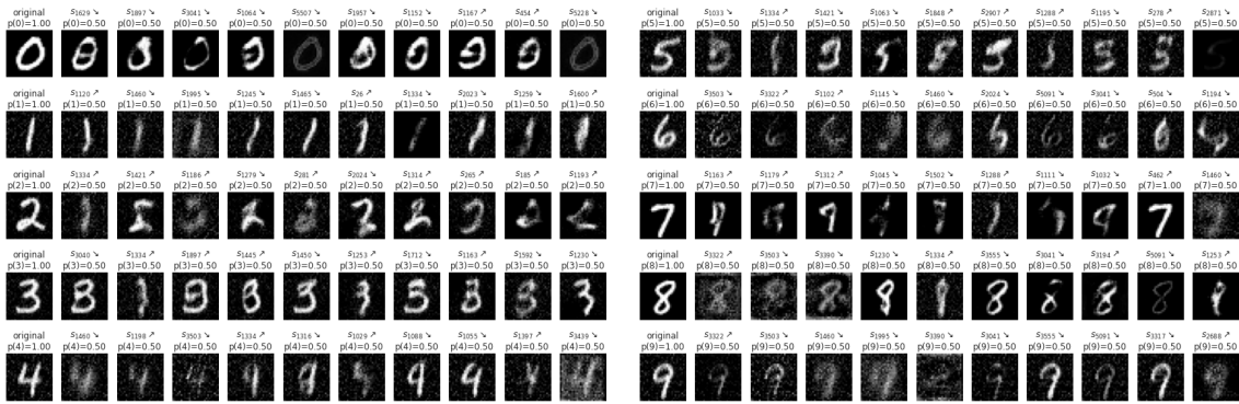
Figure 3.8: Illustration of extreme examples found for each class. By starting from the average image in StyleSpace for the class, its latent code in one of the top ten influential dimensions is modified until the classifier shifts its prediction (softmax probability for the given class falls to 0.50). Above the images are displayed the StyleSpace dimension index, an arrow representing the direction to follow (augment or reduce the value), and the classifier output for the true class.
