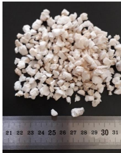
Figure 2. Sunflower pith used to manufacture particleboards.
