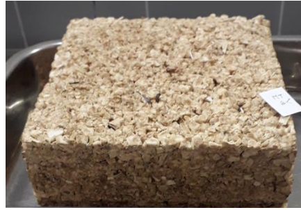
Figure 1. Particleboards made of sunflower pith (no binder)
