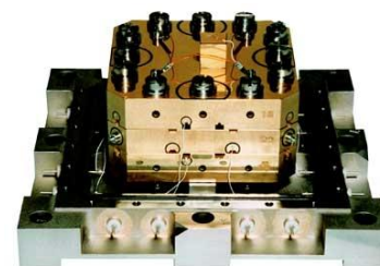
(b) STAR electrostatic accelerometer of the CHAMP mission .
