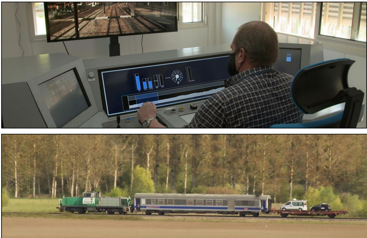
Figure 14 TC-Rail's demonstrator of a remotely controlled train, 2021
