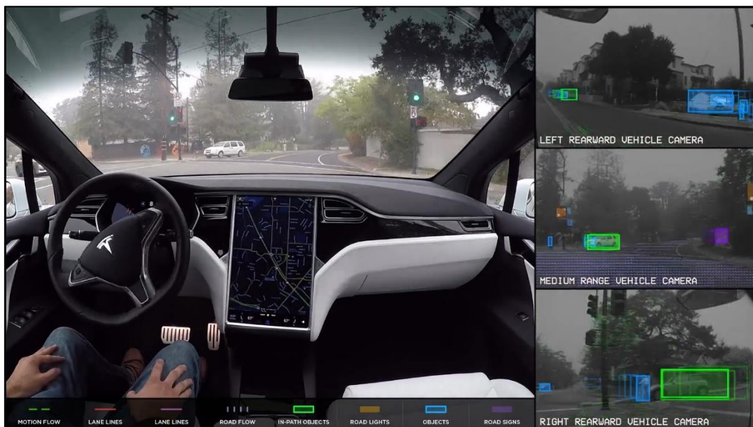
Figure 1 Tesla autopilot with continuous objects detection from cameras (from Tesla promotional pictures)
