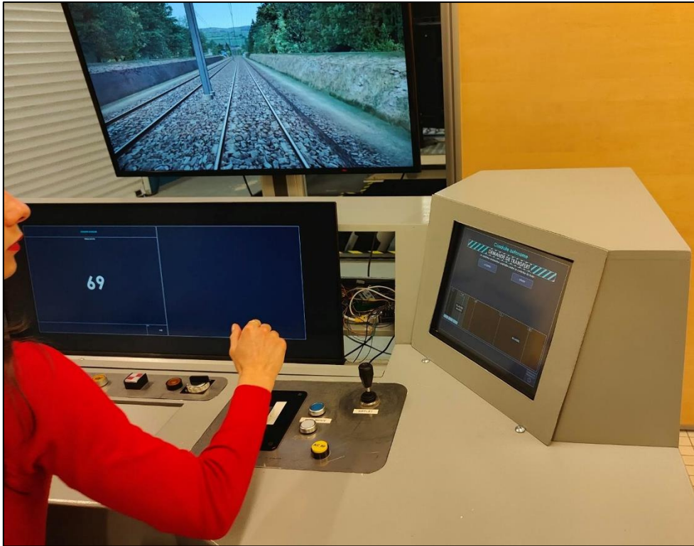
Figure 68 Remote driving platform in use: TOR from the virtual interfaces
