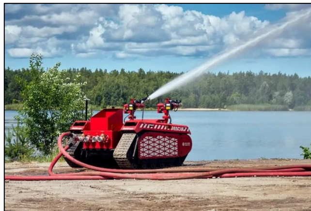
Figure 12 Milrem's "Multiscope Rescue with Hydra, a firefighting UGV
