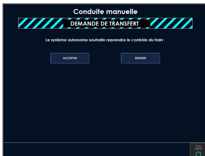
Figure 51 Transfer assistance panel example: Autonomous train issues a TOR to switch to autonomous driving
