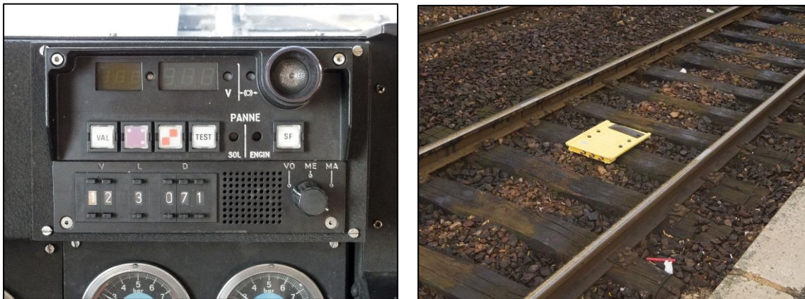
Figure 5 In-cab KVB display and KVB beacon on the rails
