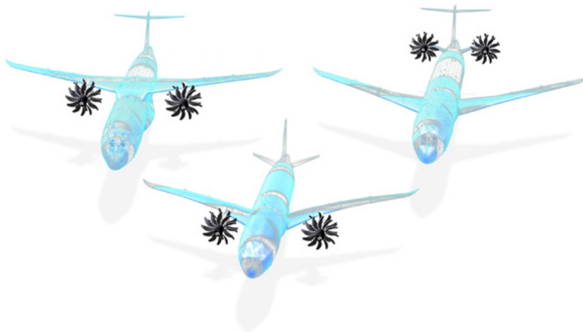
Figure 1.8: UDF engine installation [SAE-GE, 2021].
