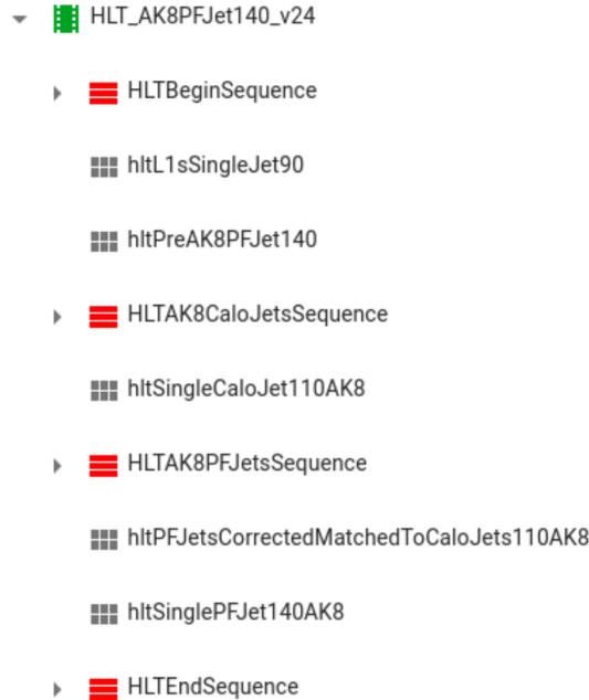
Figure 3.1: General structure of the HLT path HLT_AK8PFJet140_v24 obtained with the ConfDB database [235].
