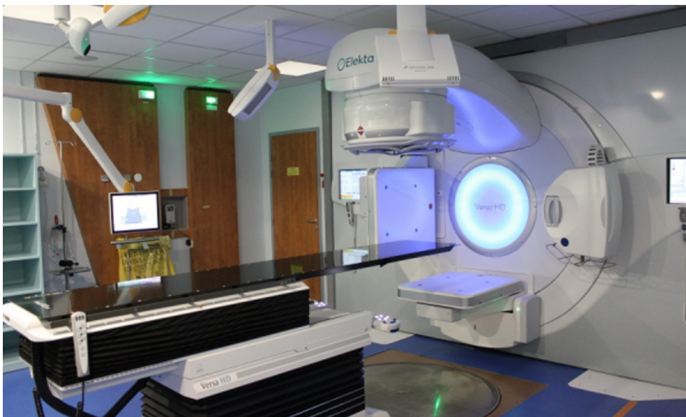
Figure 2.2: The Elekta Versa HD system with Cone Beam CT (CBCT) imaging. The CBCT provides 3D anatomical visualization by performing a complete gantry rotation around the patient.
