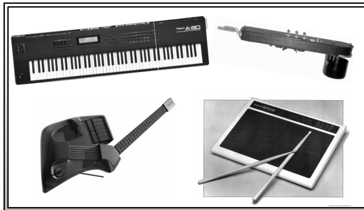
Figure 2.1: Roland A-80, Nyle Steiner EVI, SynthAxe, and Roland SPD-8 are MIDI controllers that afford interactions transferred from acoustic physical instruments.
