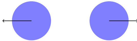
Figure 2: Two charged droplets repelling each other because of electrostatic forces.
