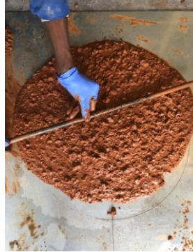
Fig. 71. Measuring slump flow diameter of concrete.
