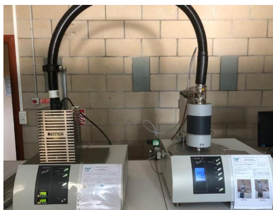
Fig. 80. Netzsch machine model STA 449 F3 Jupiter + QMS Aeolos 403 °C.
