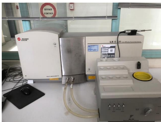
Fig. 52. Laser granulometry using LS 13320 Beckman Coulter.
