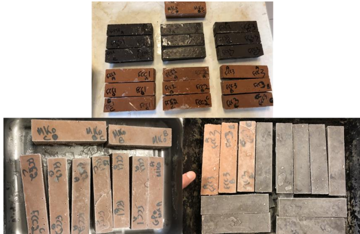
Fig. 75. GP mortar samples upon freeze-thaw test.
