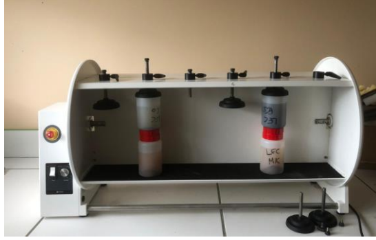
Fig. 83. Leaching test on designed formulations.
