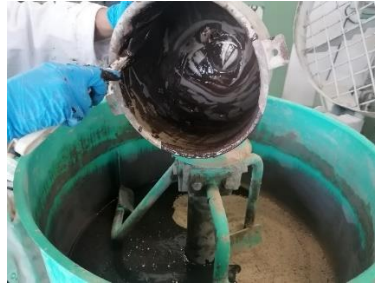
Fig. 69. Concrete mixing procedure.
