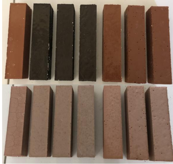
Fig. 120. Visual inspection of GP formulations before and after conducting the high-temperature resistance test.
