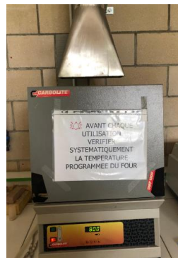
Fig. 76. Oven used for high-temperature resistance test.
