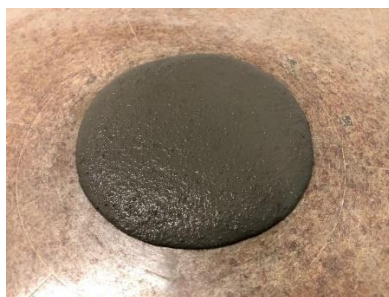
Fig. 70. Measuring slump diameter using flow table.
