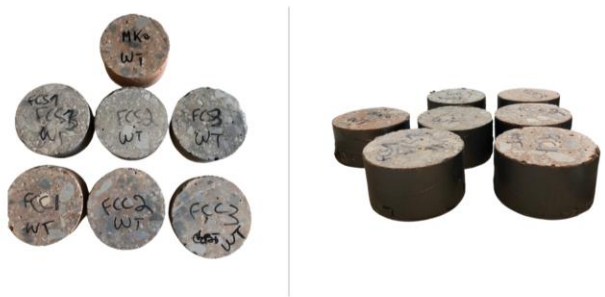
Fig. 77. Concrete specimens before and after sealing.
