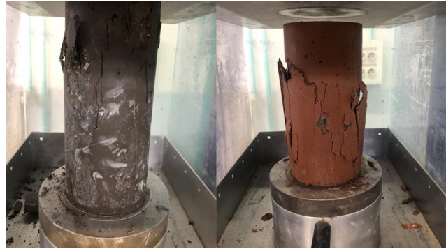
Fig. 73. Examples of concrete cylinders after compressive strength test.
