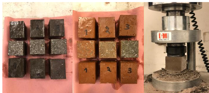
Fig. 72. Compressive strength on mortar formulations.
