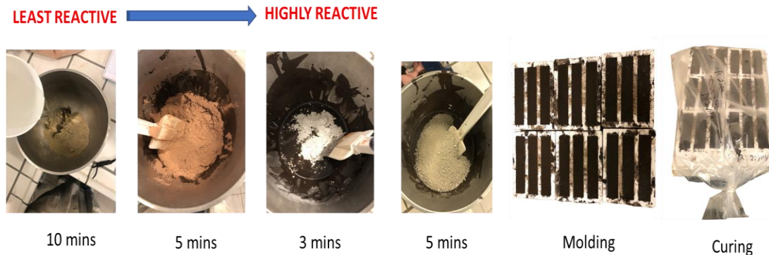
Fig. 67. GP mixing procedure.
