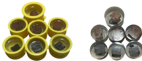
Fig. 78. Samples preparation for SEM.
