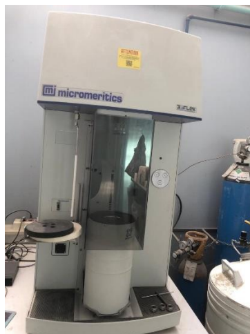
Fig. 51. Measuring BET using 3FLEX 3500 flex.
