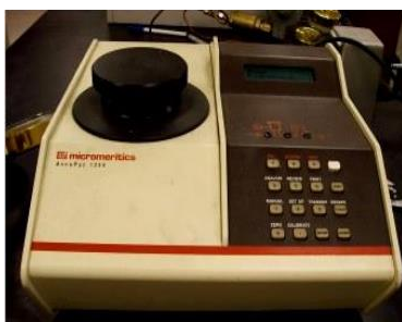
Fig. 50. Helium pycnometer to measure materials' absolute density.
