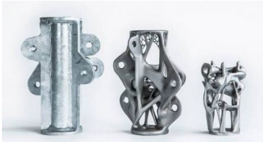
Figure 1.21 – Topology optimization achieved through AM. On the left, TM piece, while moving on the right, more complex products, increasing miniaturization through AM (from [25]).
