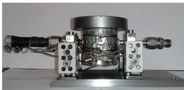
Figure 2.4: Profil view of the inlet system for sample removed from the vacuum chamber of experimental device CLUB.
