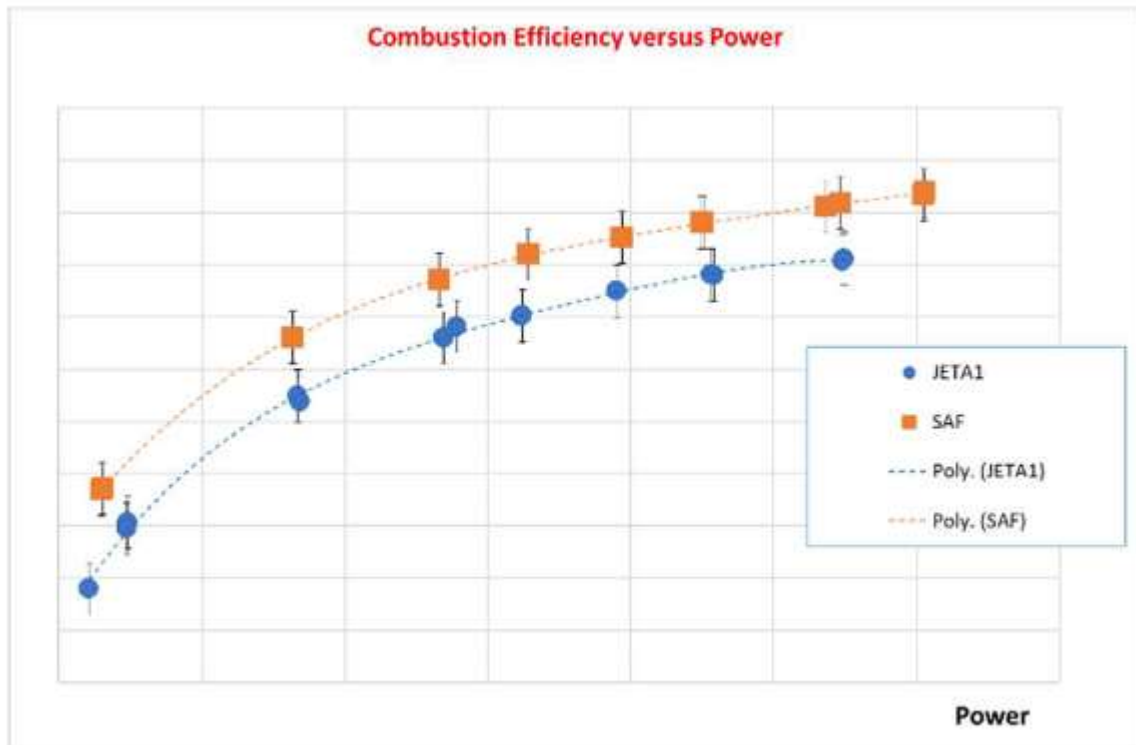
FIGURE 104 combustion efficiency vs engine power for SAF (red) and CAF (blue), source Jean-Baptiste Jarin and Jean-Louis Champion
