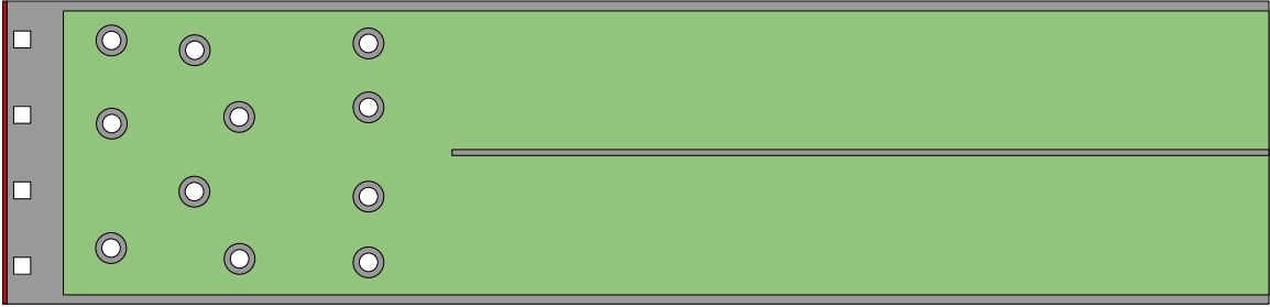
Figure 2.1: 2D WCLL domain showing W ■ , Eurofer ■ , PbLi ■
