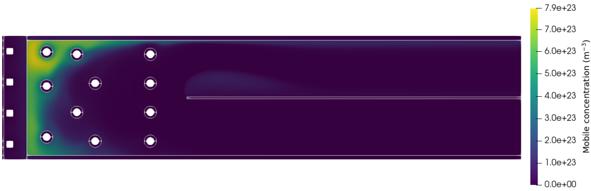
Figure 3.13: Tritium mobile concentration, c_m , field at steady-state
