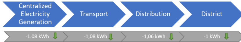
Figure 13: Transport and distribution of 1 kWh marginal electricity from the national power system
