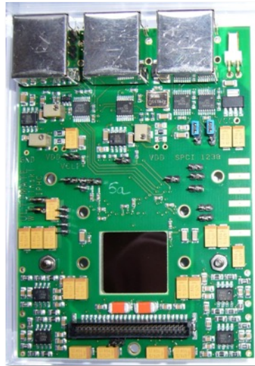
Figure 2.8: MIMOSA-28 CMOS pixel sensor photo
