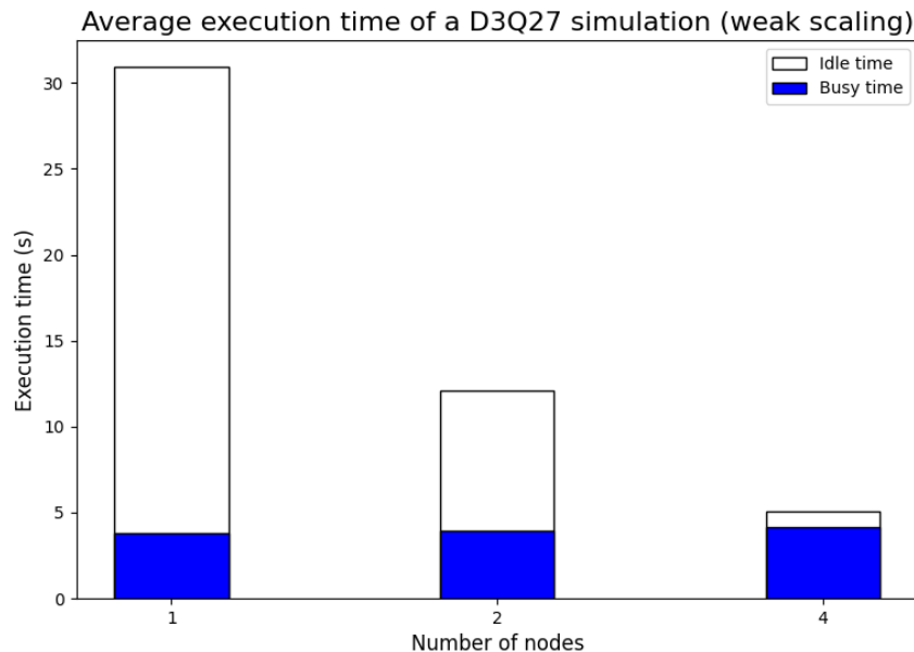
Figure 5.7: Weak scaling of the StarPU implementation of the D3Q27 scheme. The total grid size increases with the number of nodes.
