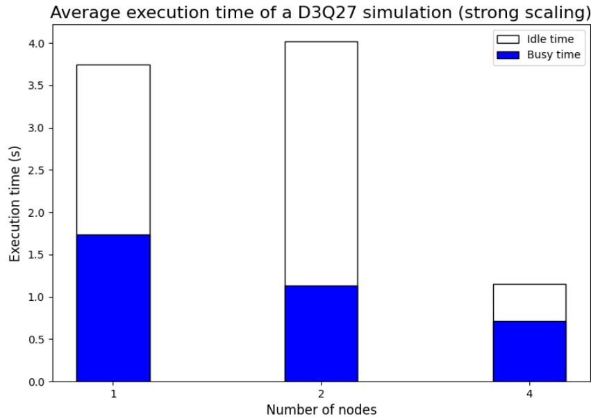
Figure 5.6: Strong scaling of the StarPU implementation of the D3Q27 scheme. The total grid size is fixed and the number of nodes is increased.
