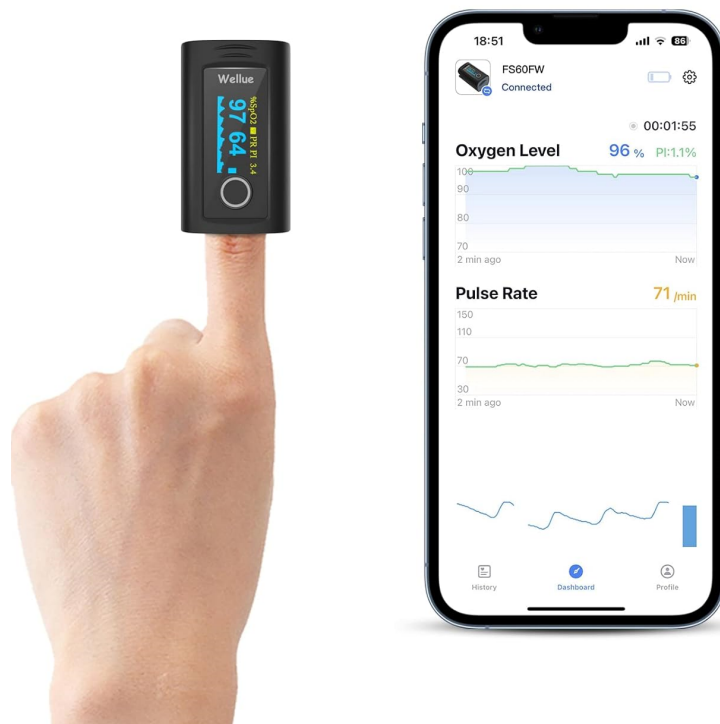
Figure B.1 – Left: Oximeter used to record the heart rate beats of the students. Right: ViHealth application that receive the data from the oximeter.
