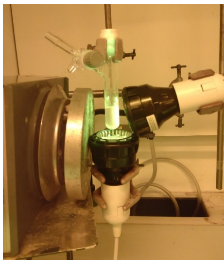
Figure S20: Photocatalytic set-up for imine synthesis under nitrous oxide atmosphere.
