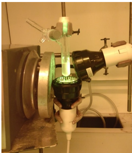
Figure S18: Photocatalytic set-up for phosphines oxidation under nitrous oxide atmosphere.
