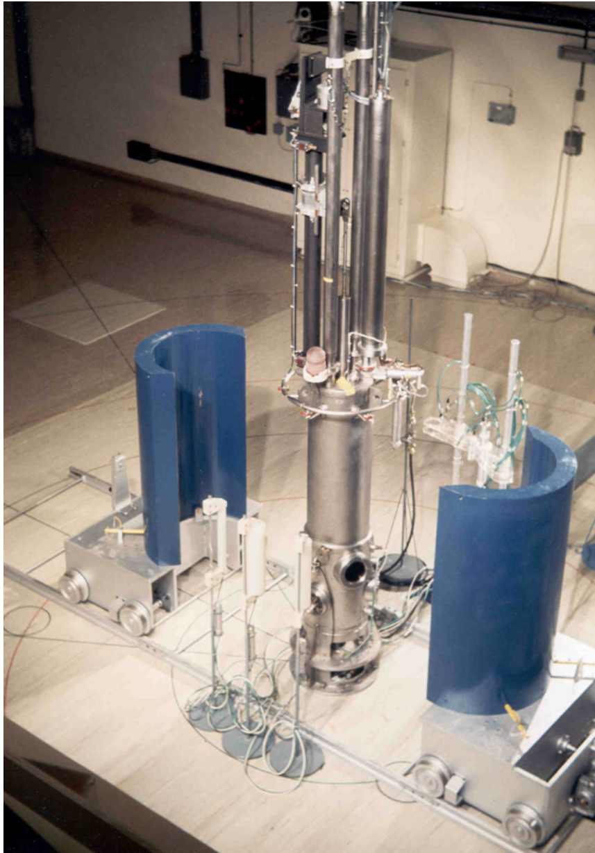
FIGURE A.4: Photograph of the SILENE core with steel reflectors.
