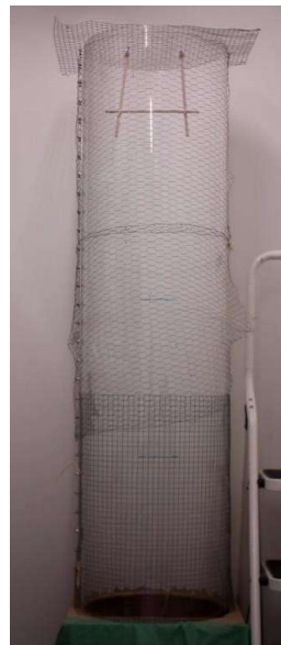
Figure 2. Tube used for flying test. The bird is put in the bottom through the curtain and startled by clapping, making it fly up to the top perch. The speed is then calculated by the number of frames spent between the marks.
