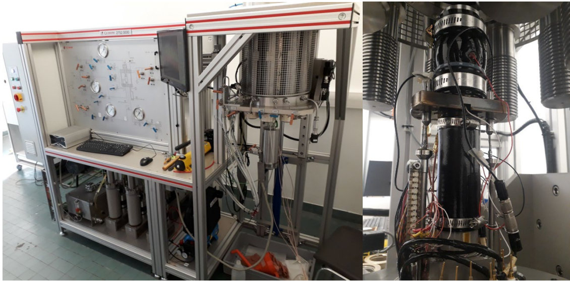
Figure 4.1: Top Industry triaxial cell: (left) when cell is closed, (right) cell is open, close up on jacketed sample. Modified after Borgomano et al., 2020;
