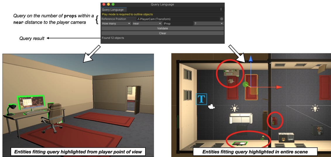
Figure 3.8 – Here we show the window to construct a simple query using the syntax from Figure 3.4 that counts the number of props within a near distance (3 meters) of the player camera. The two views show the highlighting in the scene from the player viewpoint (left) and the Unity scene view from above (right).
