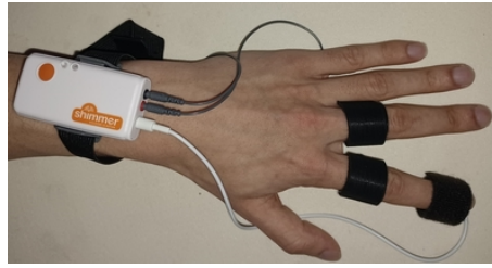
Figure 4.1 – Shimmer3 GSR+ used to record EDA and optical pulse. Gray wires connect the EDA sensor, white wire connects the pulse sensor.
