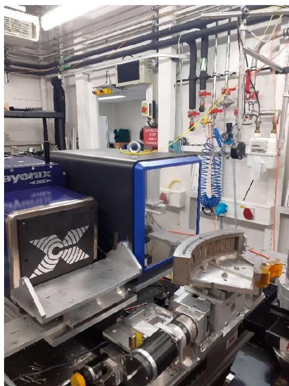
Figure 3.10. Eiger2X CdTe photon-counting detector from DECTRIS on the right and rayonix MX170-HS detector on the left.
