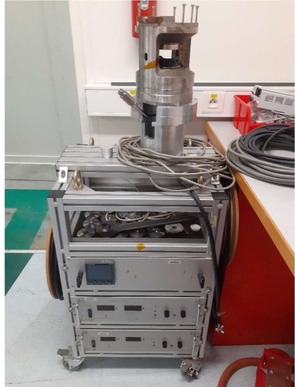
Figure 2.10. Photographs of the pressure generator (left) and the power supply with the PEP (right).
