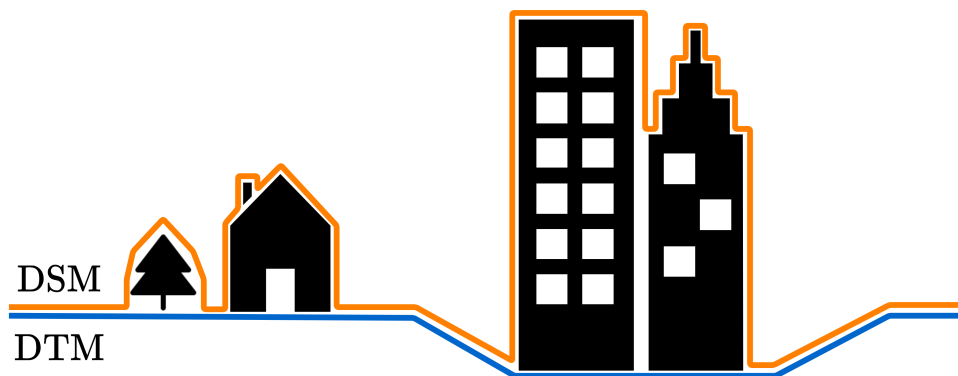
Figure 1.1: Difference between Digital Terrain Model and Digital Surface Model
