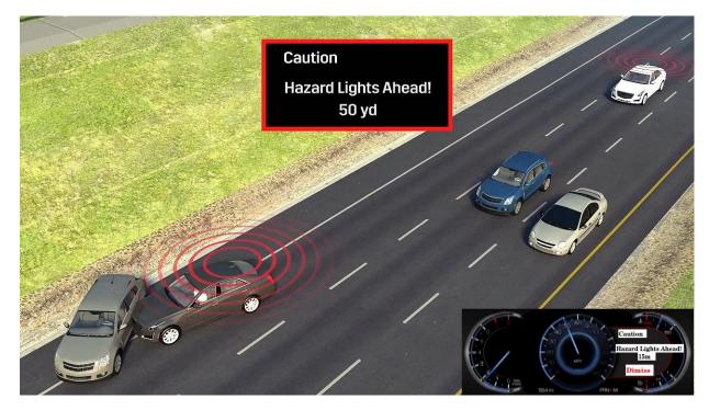
FIGURE 2.2 – Crash detection through V2V communication[1]
