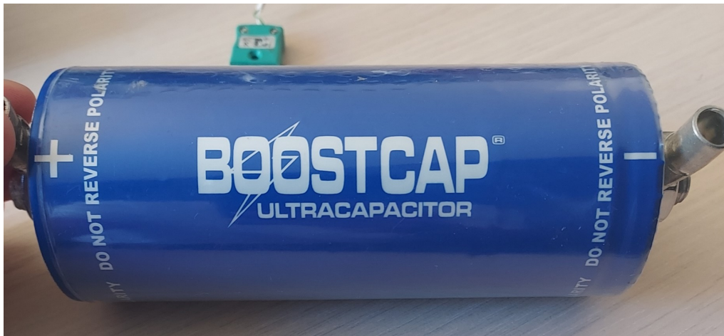
Figure 3.21 – Supercondensateur Maxwell 2600 F
