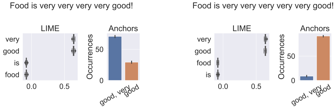
Figure 3.3 – Making a word disappear from the explanation by adding one occurrence. The classifier \mathbb{1}_{(very \in z \text{ and } good \in z)} is applied when m_{very} = 4 (left) and m_{very} = 5 (right).
