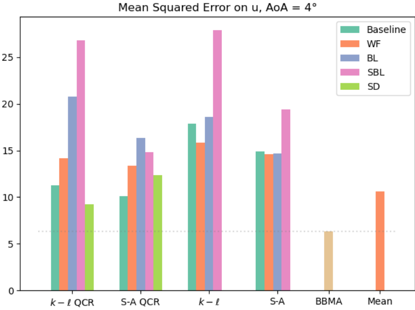
Figure 7.19 – Mean squared error on longitudinal velocity for baseline and updated models and the BBMA trained on scenario 4DEG
