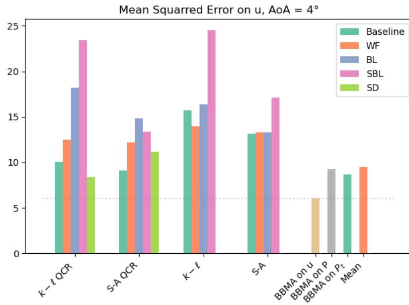
Figure 7.23 – Mean squared error on longitudinal velocity for baseline and updated models and the BBMA on various quantities and mean reconstructions after calibration and weighting on scenario 4DEG
